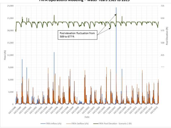
Figure 3.5 FRFA Operations Modeling – Water Years 1989 to 2015
