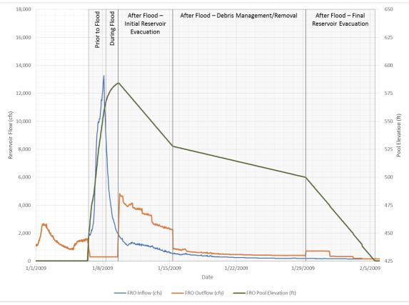
Figure 2.8 FRO Operation Modeling – January 2009 Flood
