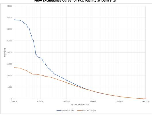
Figure 2.9 Flow Exceedance Curve for FRO Facility at Dam Site
