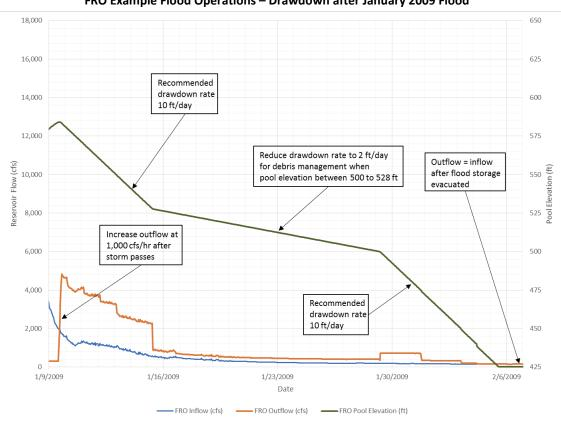
Figure 2.3 FRO Example Flood Operations – Drawdown after January 2009 Flood
