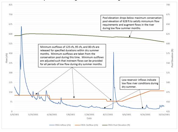
Figure 3.7 FRFA Operations Modeling – Minimum Flows During Summer 2001
