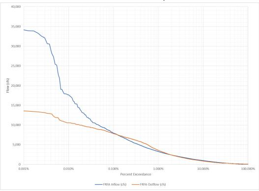
Figure 3.11 Flow Exceedance Curve for FRFA Facility at Dam Site
