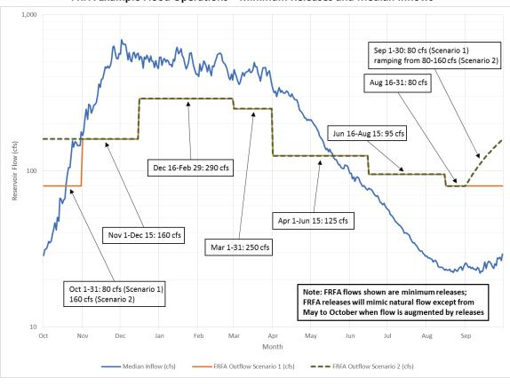
Figure 3.3 FRFA Example Flood Operations – Minimum Releases and Median Inflows
