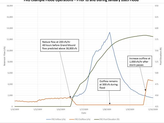
Figure 2.2 FRO Example Flood Operations – Prior to and During January 2009 Flood
