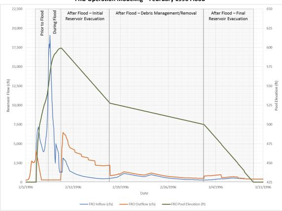
Figure 2.6 FRO Operation Modeling – February 1996 Flood
