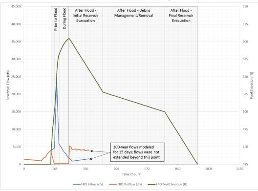
Figure 4.1 FRO Flows and Elevations – Current 100-year Flood
