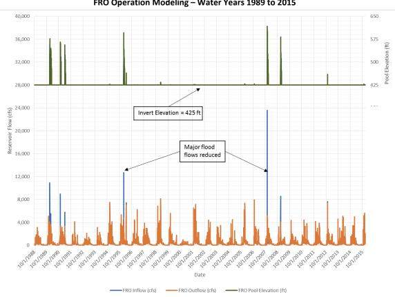
Figure 2.5 FRO Operation Modeling – Water Years 1989 to 2015
