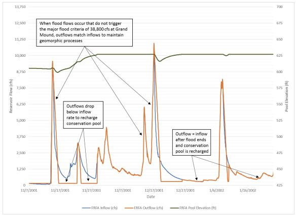
Figure 3.1 FRFA Hourly Flows and Elevations – Frequent Flooding Operations
